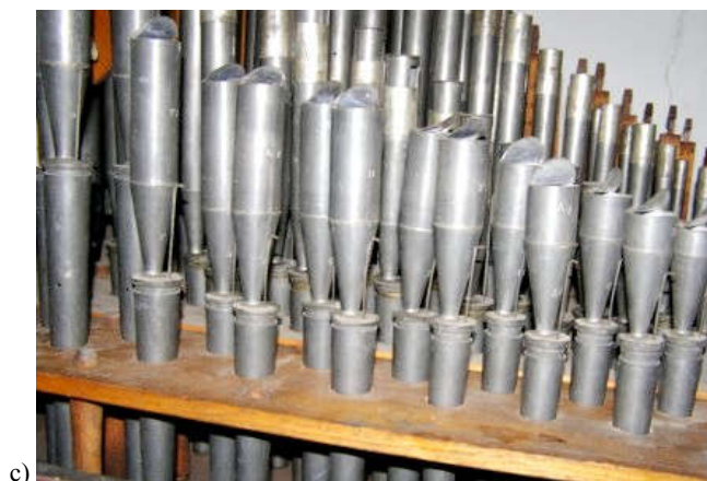
Figure 2. Pipe examples of Type 1: a) Vox humana drawings (left – Bédos, 1766, engraving No. 18, fig. 141; right – Audsley, 1905, fig. CCCLVI); b) Trompet pipes in Kretinga Franciscan Church (unknown master, end of the 17th c.; Lithuania); c) newly manufactured (2008) Vox humana pipes of this type for the organ in St. Paul’s Stoneycroft, Liverpool (UK).
